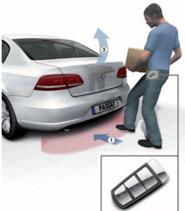
4 Opening (2) the boot lid by detection of foot motion (1)
