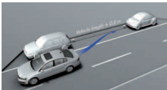
11 Easier parallel parking (left) and diagonal parking (right) with the Park Assist
