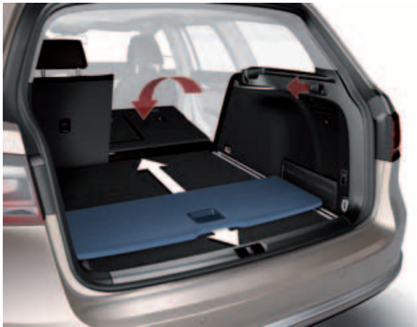
5 Remote rear seat backrest unlatching from the luggage compartment
