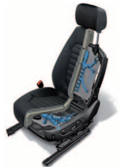
7 Active front seat ventilation with radial fans and air ducts in the foam upholstery
