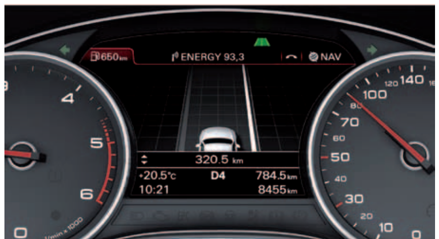
② System status (green LED) and detected road markings on central display: two road markings detected (top), one road marking on the right detected (bottom)
